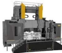
Double-column vertical turning and boring lathe
