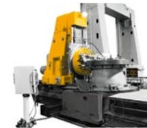
Gear milling vertical-type machine
